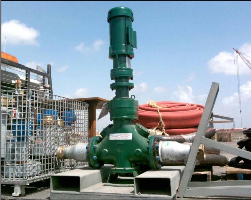
*T&T mounts the Monster grinders on a portable skid so it's easy to store and quick to deploy when vessels are handling liquids with lots of debris.*
