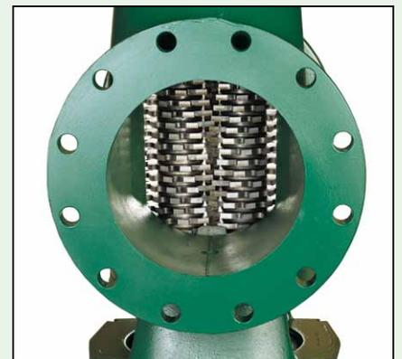
***Two shafts of sharp steel cutters cut trash and debris into particles to keep pumps, valves and pipes from clogging. The grinder bolts right into almost any pipeline – from 4" (100mm) and up.***
