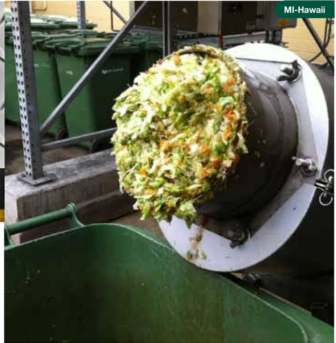
*Shredded and compacted food waste is dropped into the disposal bin.*
