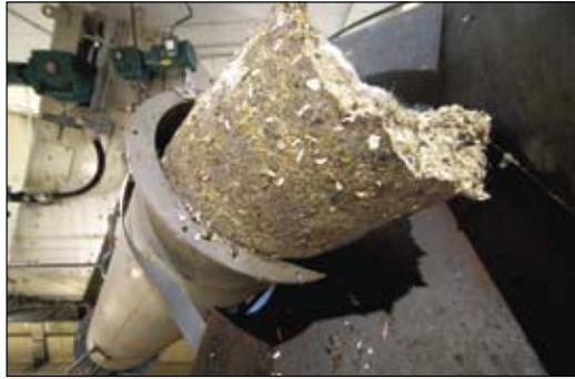
**Adding a grinder to a washer–compactor can lead to cleaner, more compact screenings for disposal. A head-to-head comparison by the Greater Vancouver (British Columbia) Regional District laboratory showed fecal coliform rates four times higher in screenings that did not pass through a grinder than in those that did.**
