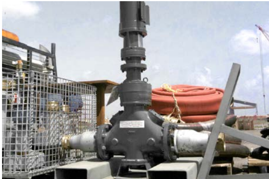
T&T mounts the Monster grinder on a portable skid so it's easy to store and quick to deploy when vessels are handling liquids with lots of debris.
