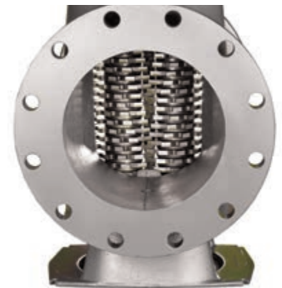
Two shafts of sharp steel cutters cut trash and debris into particles to keep pumps, valves and pipes from clogging. The grinder bolts right into almost any pipeline – from 4 inches (100 mm) and up.
