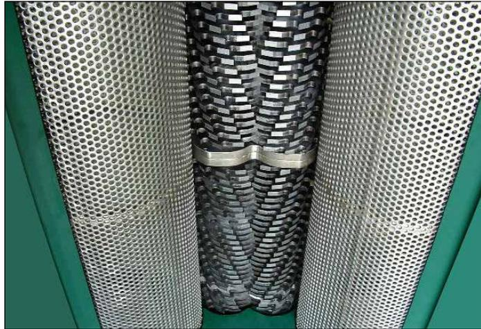
*High-flow screening drums capture solids and direct them into the grinder*
