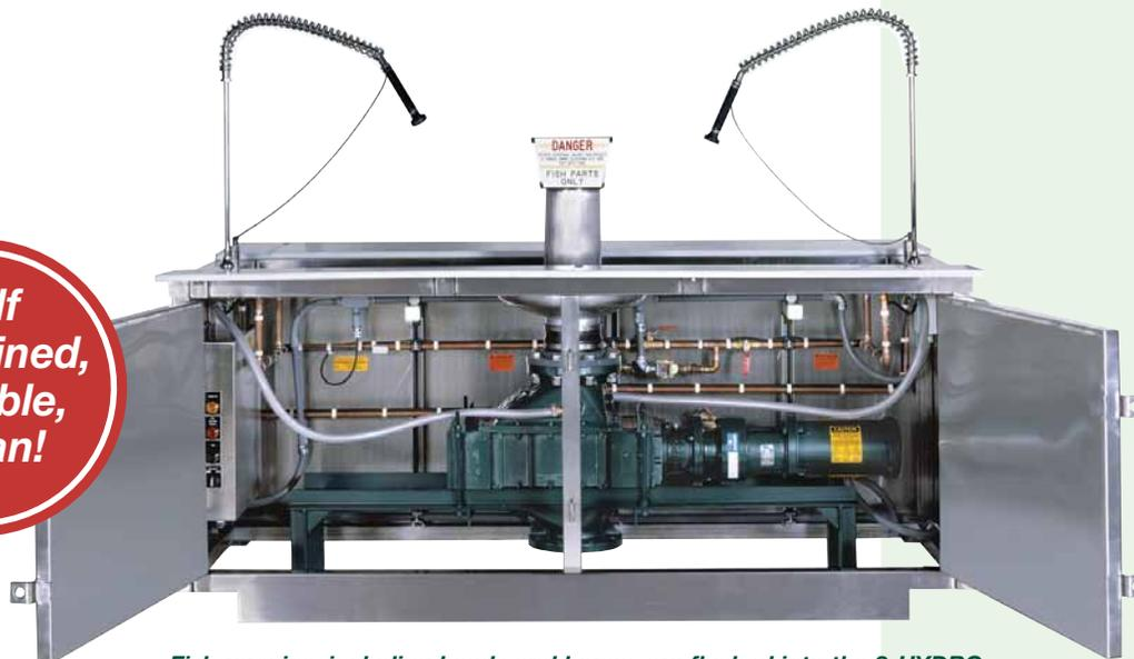
*Fish remains, including heads and bones, are flushed into the 3-HYDRO grinder by two water streams. Ground up remains are quickly washed away.*
