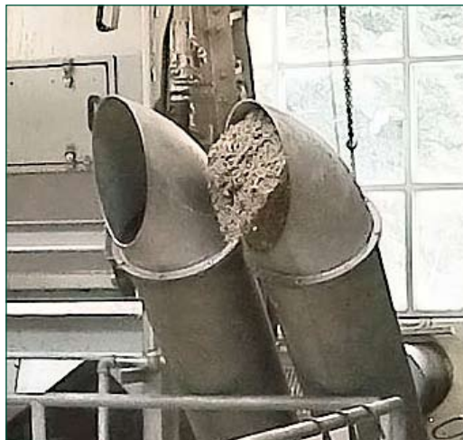
The SWM's grinder and two spray wash zones produce cleaner, drier discharge.
