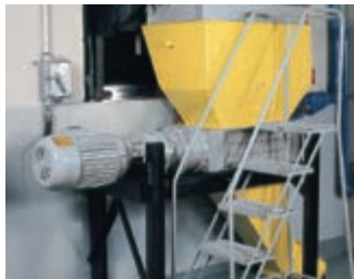
4-SHRED-H with custom hopper and discharge chute
