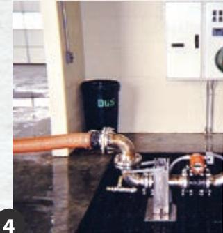
4 The operator connects and locks on the discharge hose and unloading begins.
