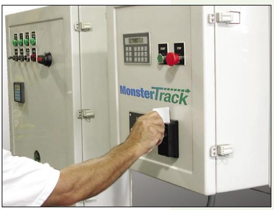
Automated MonsterTrack PLC Controller allows easy sign-in and operation of the Honey Monster, saving time and paperwork for truck drivers and the billing office.
