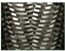
The powerful dual shafted cutters destroy items in one pass without jamming
