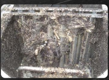
The screening bars use a unique design for max flow while capturing silverware, rags and plastics. A hot water washdown cleans the bars.
