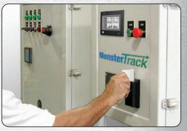
MonsterTrack billing controller features a card lock and receipt printer.
