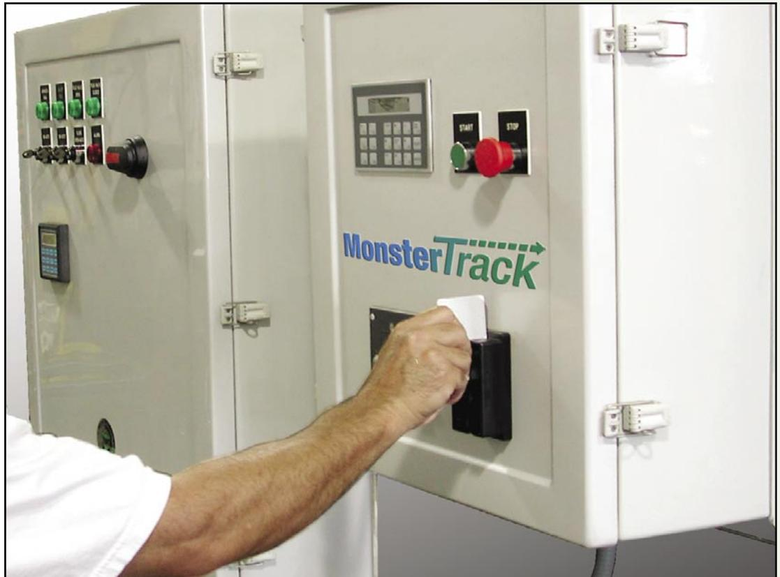
***Automated MonsterTrack PLC Controller allows easy sign-in and operation of the Honey Monster, saving time and paperwork for truck drivers and the billing office.***
