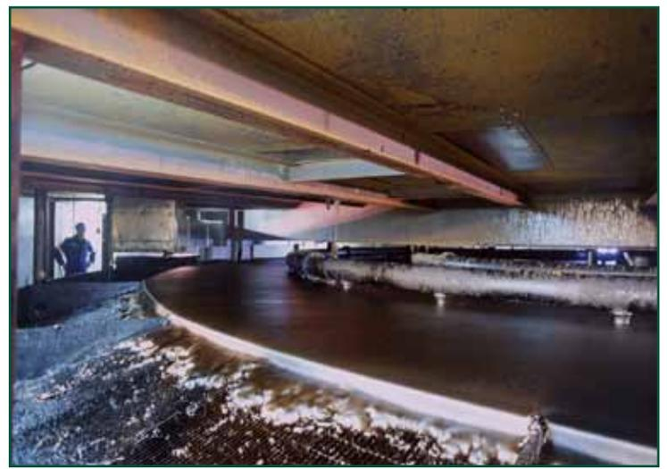
Here, raw bitumen is separated from the sand in Suncor’s giant separation cells.
