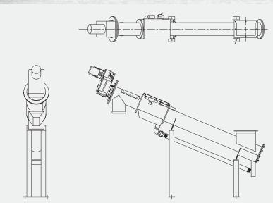
The capacity of the PLT may vary due to characteristics of the solids material and the slope of the unit.
