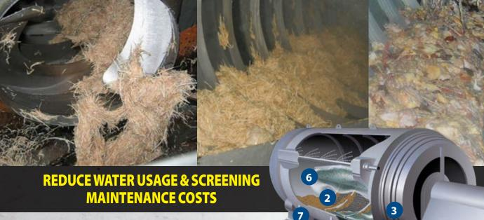
The IFO, IFU and IFS series of internally fed rotary drum screens have cylindrical drums mounted horizontally on four shaft-mounted wheels. The drum rotates at 4-5 rpm and is driven by a TEFC motor, geardrive, chain and sprocket.
