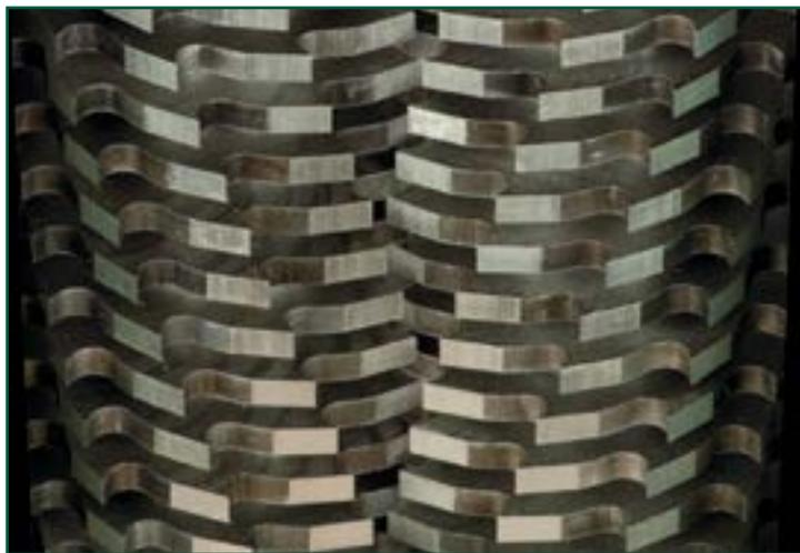
*A Monster sewage grinder has two rows of sharp, steel cutters that rotate slowly and at high-torque.*
