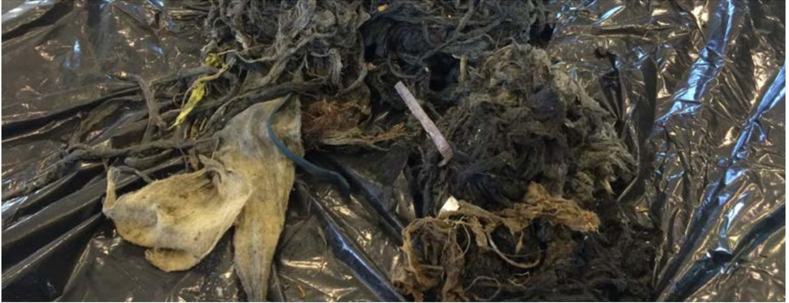
twine together and build up in the wet well. “The grinders were doing their job, but this material just doesn’t dissolve,” said Gary Burrows, operations supervisor for the City of London. “We were having an insurmountable amount of rags weaving in our wet wells.”
