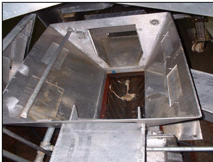
Muffin Monsters readily grind up the many types of seafood remains conveyed into its specially designed cutter teeth.
