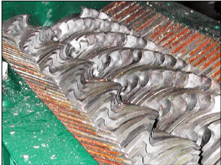
The specially designed cutters can slice through a 200lb. (90 kg) halibut and turn it into puree within seconds.
